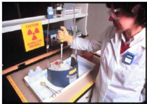
Figure 18 Use of Plexiglas Shielding
